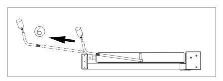
6. Remove the bottle of lubricant and the applicator tube. The message "PLEASE PRESS THE STOP KEY AFTER FINISHING LUBRICATION" appears. Press the STOP key to stop the walk belt and exit the lubrication mode.
