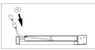
4. Squeeze 50cc of HyperGlide<sup>™</sup> lubricant out of the bottle and into the applicator tube.
