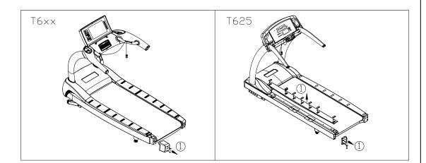
1. On T630, T650, T650M, T670, T680 treadmills, remove one end cap (left). On T610, T620, T625 treadmills, remove one end cap and one landing strip (right).
