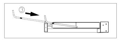
3. Insert the lubrication applicator tube so the line on the applicator tube touches the edge of the walk belt.
